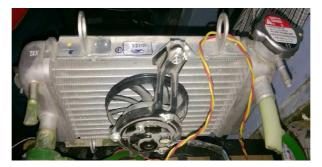
Figure 2: Radiator and Radiator Fan
